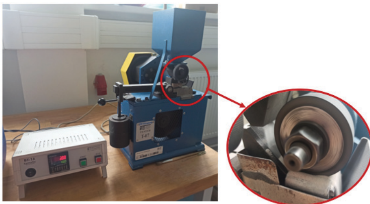
Fig. 2 Device for testing according to GOST 23.208-79 with detail Obr. 1 Prístroj pre skúšku podľa GOST 23.208-79 s detailom
