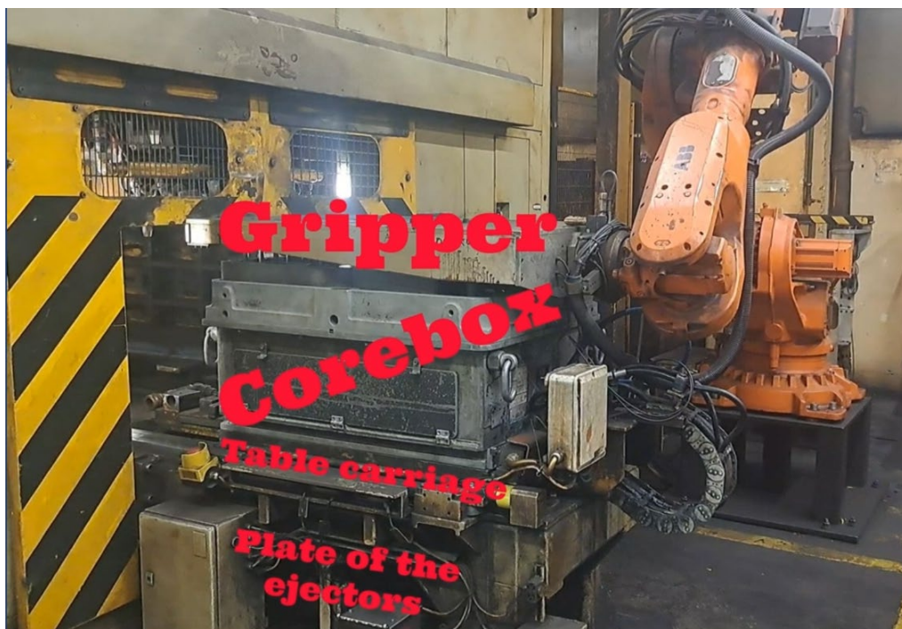
Fig. 1 Removing cores from the mold using a robot with an effector
