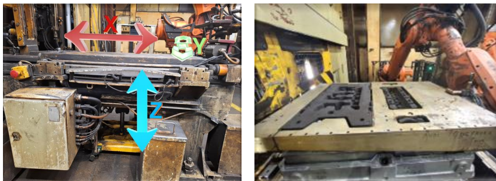
Fig. 6 Press imperfections in the X, Y and Z axes (left) and the manipulator removing sand cores from the press (right)
